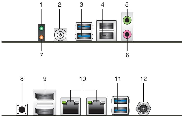
1. **Power LED.** This power LED lights up when you turn on the Slot-In PC.
