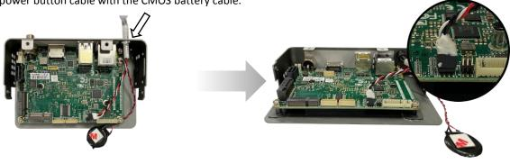
**Step 6:** Peel the backing off of the tape on the CMOS battery. Gently press the battery onto the PICO-APL3 board to secure it.
