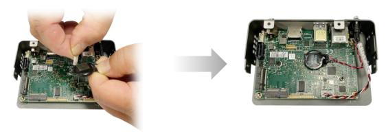
**Step 7:** Attach the bottom chassis by first lining up the right side, then swivel the chassis into place. NOTE: the bottom chassis does not slide directly on, it must swivel into place as shown in the figure.
