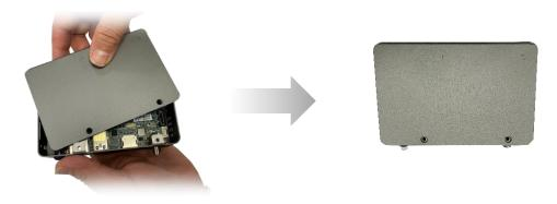
**Step 8:** Ensure the bottom chassis is properly lined up and attached. Use black screws to secure, two screws on the bottom and one screw on the left and right sides of the chassis.
