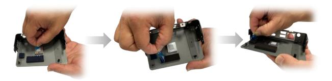
Step 2: On the PICO-APL3 board, remove the nut and washer from the power input port.
