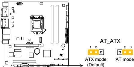
**IMBM-H110A H/W AT/ATX mode selection**
