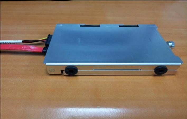
Step 8: Turn the screw counter-clockwise to secure the casing
