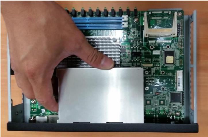
Step 3: Turn screw clockwise to open HDD casing
