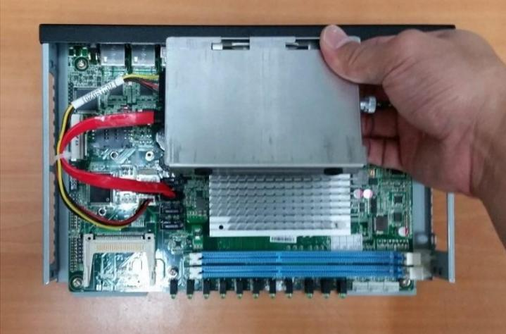
Step 10: Place the casing into the chassis, slide right to secure
