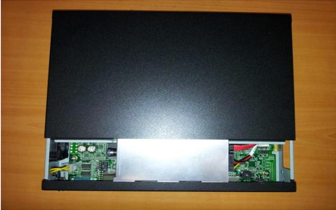
Step 2: Slide right to remove casing
