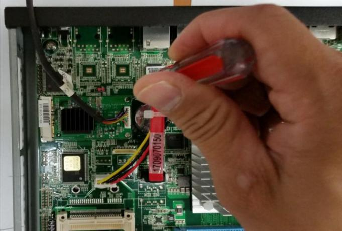
Step 4: Connect your VGA device. Both screws must be secured for the connector to function properly
