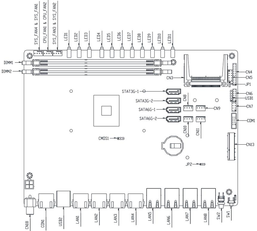
\*Memory assembly priority: (1) DIMM1 (2) DIMM2
