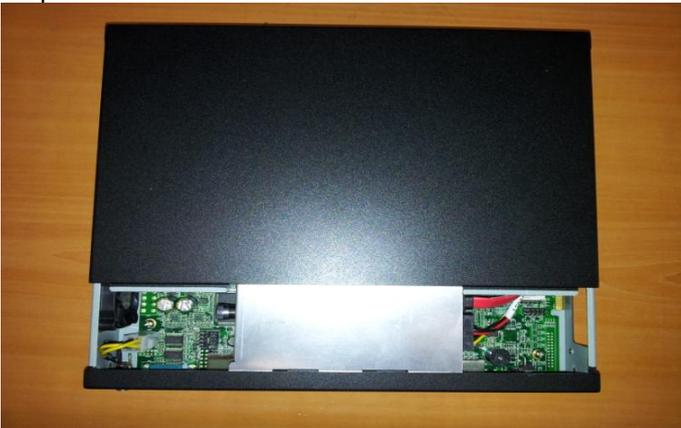
Step 2: Insert the VGA Card into Mini-PCle slot
