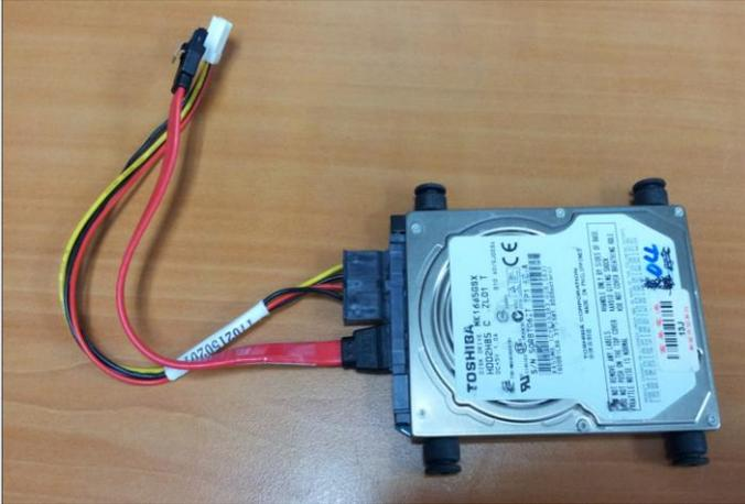
Step 6: Place the HDD onto the HDD bracket of the casing
