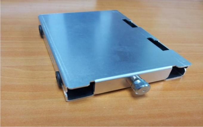
Step 4: Attach all four screws of the casing to the HDD
