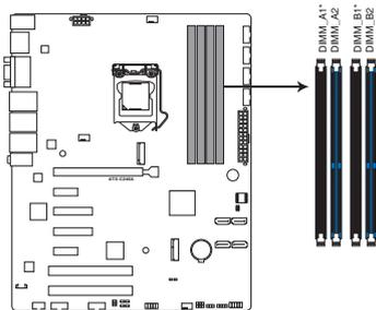
ATX-C246A 288-pin DDR4 DIMM sockets
