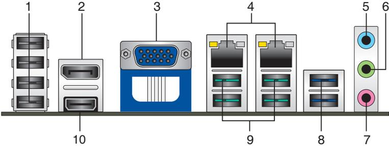
1. **USB 2.0 ports.** These two 4-pin Universal Serial Bus (USB) ports are available for connecting USB 2.0/1.1 devices.
