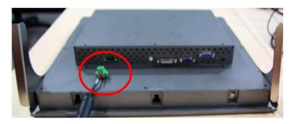
A "Surge Protection" device plugged between the AC-DC adapter and the wall outlet is recommended to prevent the effects of sudden current variations from reaching the LCD Display. The sudden peaks of electricity may harm the LCD Display.
