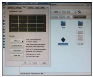
Note: If the alignments do not match display by 4 Points Calibration, please use 9 Ports or more to calibrate.
