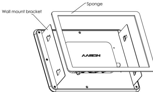
**Step 2:** Unfasten the six screws (three screws on each side respectively) and put the wallmount bracket to ACP-1103. Then, fasten the original six screws back to the ACP-1103.
