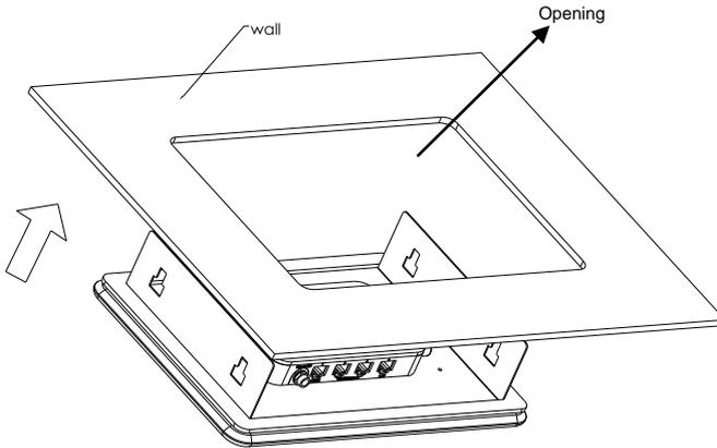
**Step 5:** Insert the mounting clips to the four fillisters on wallmount bracket and fasten the four M4x60 screws to lock the bracket
